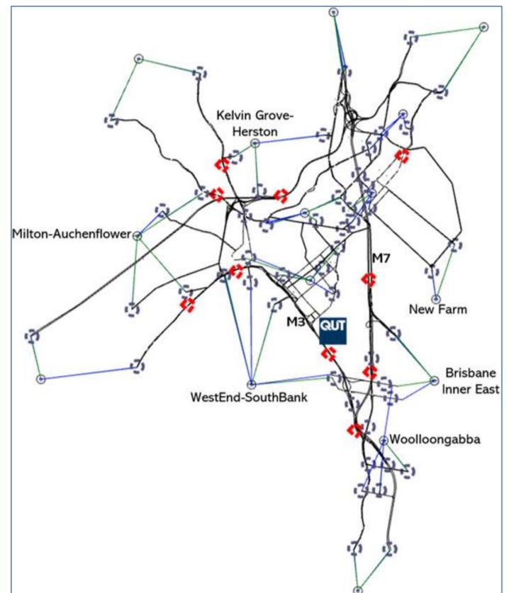
Figure 2. Network model based on Brisbane CBD. Red markers represent loop detectors and blue represent Bluetooth scanners
